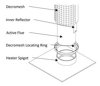
A 900mm half round inner reflector must be fitted inside the rear of the Decromesh. Using tin-snips, cut 10mm tabs into the top and bottom of the inner reflector and bend out to create an air gap between it and the outer Decromesh.
